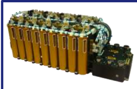
EPT part no.: SAR-10197 electrical config.: 2P9S spaceflight heritage: 8 years
