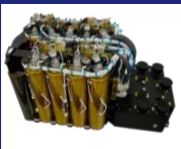
EPT part no.: SAR-10199 electrical config.: 1P9S spaceflight heritage: 7 yrs
